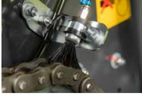
Automatic chain lubrication is standard on RF4225 Plus.
